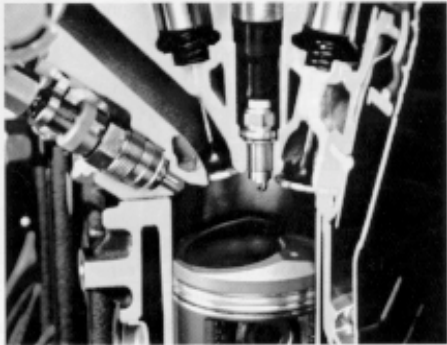
Figure 2: Cutaway view of the Toyota D4 engine showing FDI system. Source: Yamaguchi (1996)
